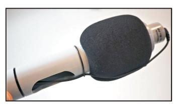
Step 6. Install one of the included O-rings onto the Mic Tube, at the location shown, to retain the 3.5mm cable.
