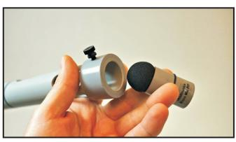
Step 2. Insert the Micro Mic PIP into the Mic Tube, wind screen first, until the O-ring is seated against the Mic Tube.
