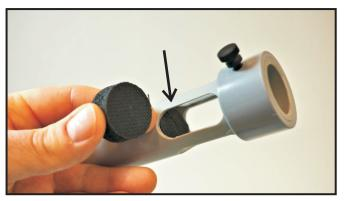
Step 1. Insert one of the foam cable clamps inside the Mic Tube as shown. This prevents resonance from the tube from effecting the microphone.
