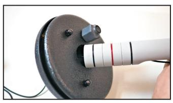
Step 8. Install the Mic Tube into the Front Plate and Back Plate that you have assembled to the parabolic dish.
