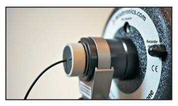
Step 9. Insert the Mic Tube so that the first black ring of the focus gauge is flush with the back of the clamp hub, as shown. Your mic is now at the focal point of the parabolic dish. Tighten the handle clamp.
