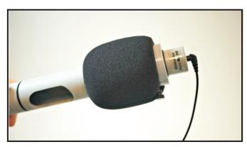
Step 4. Slide on the Windscreen, starting from the end opposite the Micro Mic PIP, until the large end touches the thumbscrew. Attach the 3.5mm cable.
